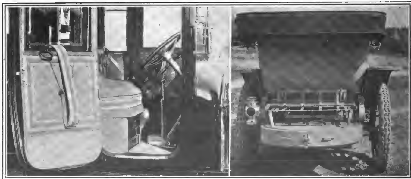
Fig. 5—Interior of the limousine and the rear of the touring model. Note tire trunk
